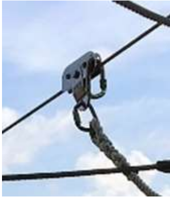
The MSR CMI Zip Line Trolley with backup steel carabiner
