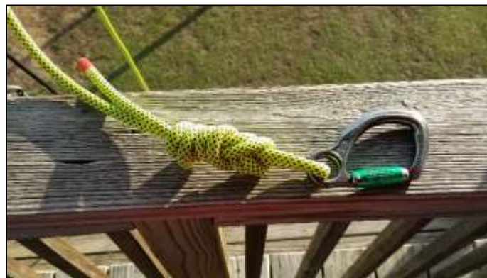
Captive eye carabiner tied with a figure 8 on a bite and properly backed up.
